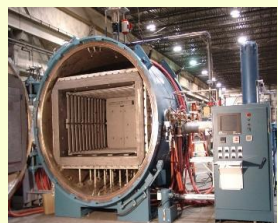
High temperature vacuum sintering furnace
