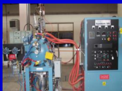
Vacuum/Hydrogen Furnace (2000°C; Gas Quenching)
