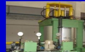
Hot Press (1050°C; under Hydrogen)
