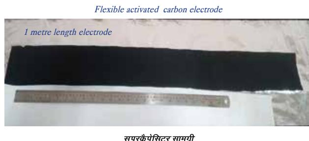
Flexible activated carbon electrode
