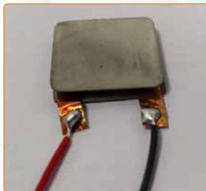
16 legs thermoelectric module and its Power – current characteristics
