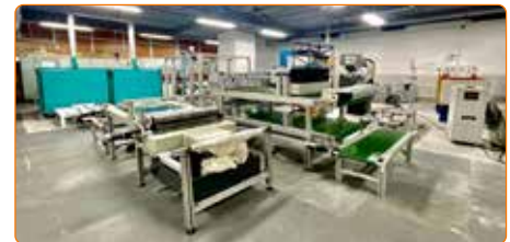
PEMFC Automated Assembly Pilot line setup at CFCT
