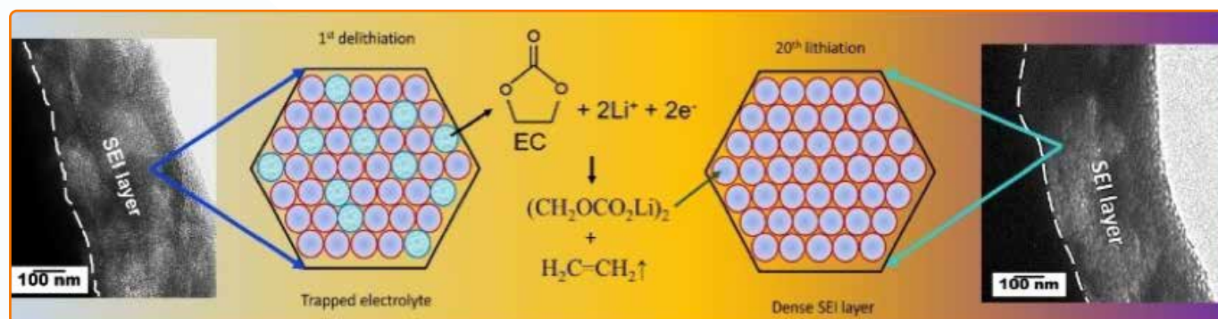
The "sponge model" of the mosaic SEI layer for initial and after cycling
