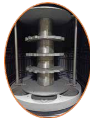
Shredder blades (mounted in vacuum system) after the TiCrN coating deposition
