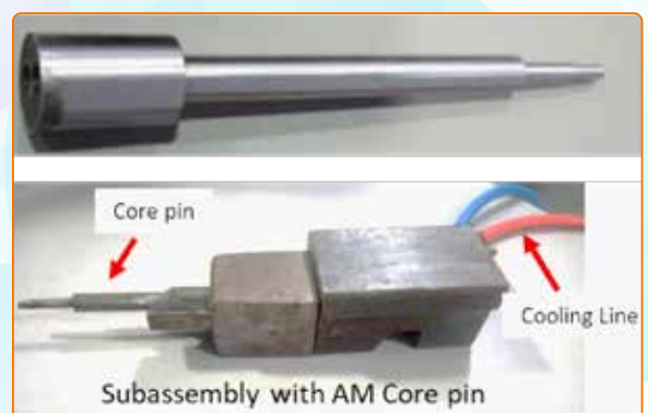
figure: Photographs showing additively Manufactured AISI H13 tool steel (a) core pin designed with conformal channel and (b) Core pin validation assembly
