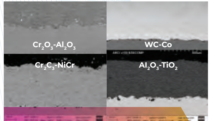
Cross-sectional images of various coatings deposited by ADSC
