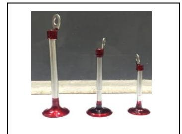
Nanocrystalline coating on Helicopter Hinge Pin (Indian Air Force)
