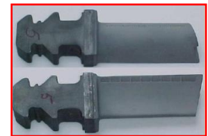
Refurbished turbine blades of power plants
