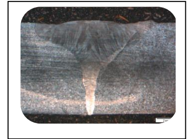
Single Pass Laser Hybrid weld cross-section
