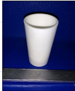
Non-oxide based green parts produced by gelcasting technique at ARCI
