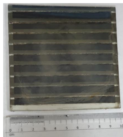
Figure: Large area carbon based perovskite solar cell
