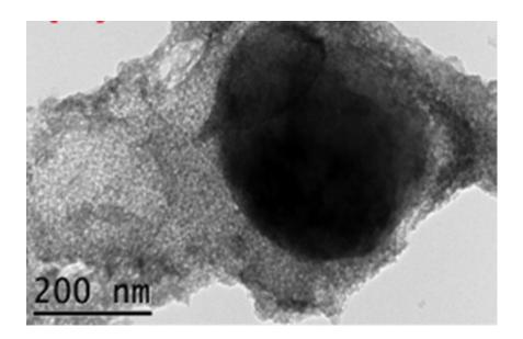
Figure Caption: Tem image of *in-situ* carbon coated  $Na_3V_2(PO_4)_3$  nanoparticles embedded in mesoporous carbon matrix.
