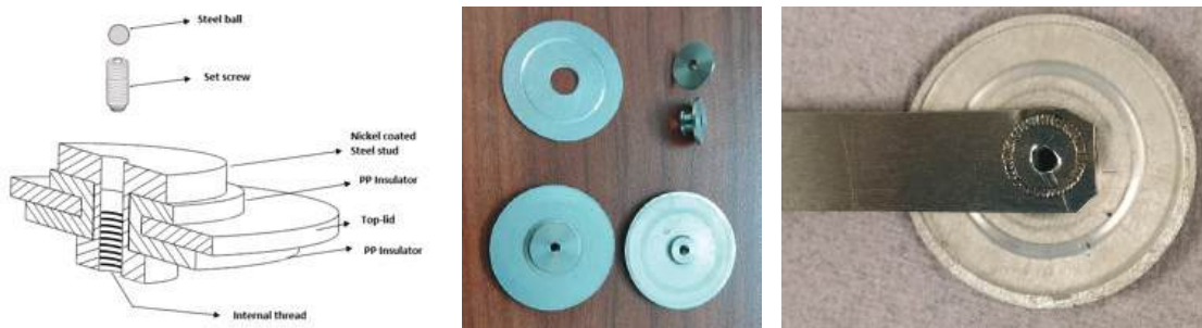
Figure 1: Novel stud-type top lid assembly setup
