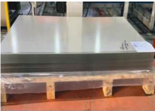
Figure 3: AR coated 1mx 2m size solar cover glass: Transmittance of Bare and AR coated glass
