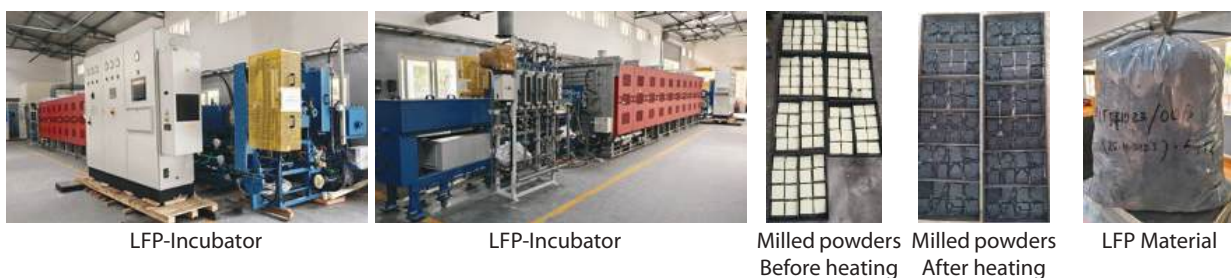
Figure: Large scale production of LFP cathode powder material by M/s. ALTMIN @ ARCI-AMTI
