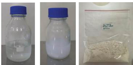
Figure 2 : a) Adhesion promoting sol; (b) Self-healing sol and (c) Self-healing additive
