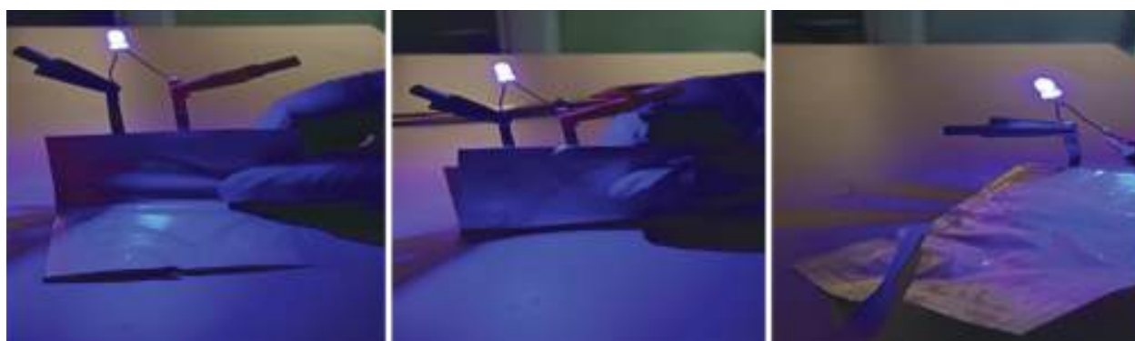
Figure 6.1: Pouch cell assembled with the QGPE - subjected to intentional abuse while under operation condition, showing no adversity.
