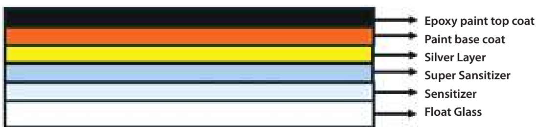
Figure 1: Schematic showing configuration of silver-based mirror
