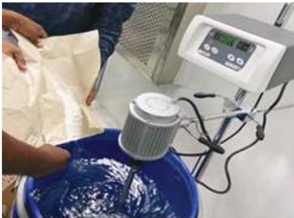
Figure 1: AR coating sol preparation in bulk quantity.
